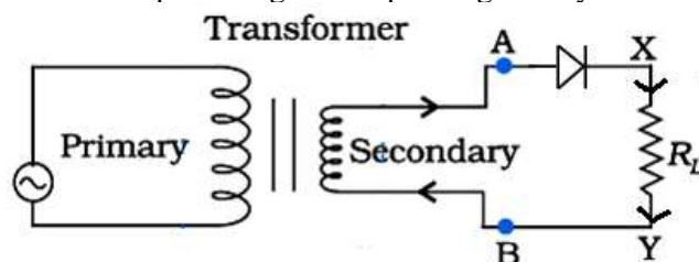
When A is positive, diode is forward biased and it conducts.
