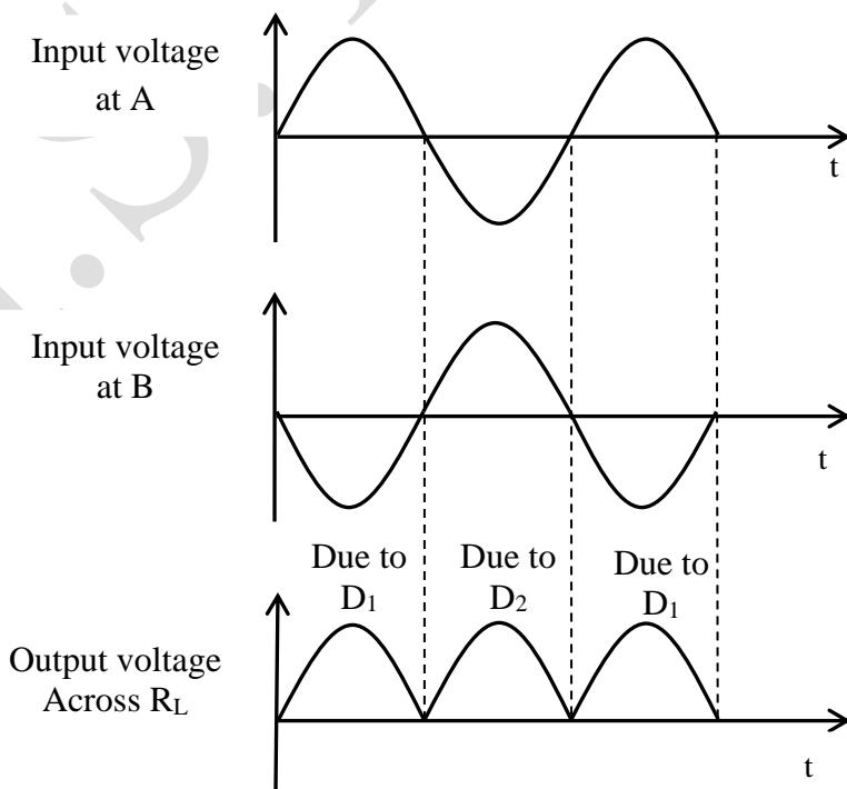
The circuit which converts ac into dc is called a rectifier.
