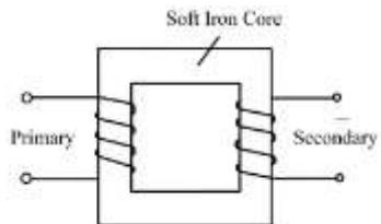
Efficiency of a transformer is given by  $\eta = \frac{\text{Output Power}}{\text{Input Power}} = \frac{V_s I_s}{V_n I_n}$
