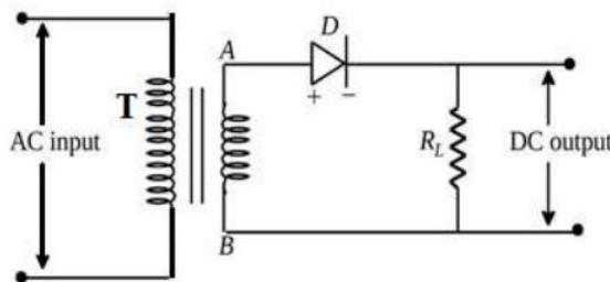
**T-transformer, D-Diode,  $R_L$  - Load Resistor** .....2 marks
