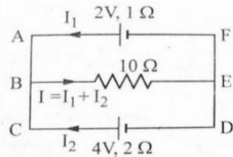
From the circuit diagram, Cells are in parallel
