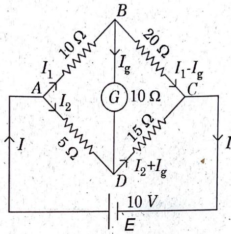
In the given Wheatstone's network, calculate the value of electric current flowing through the galvanometer.
