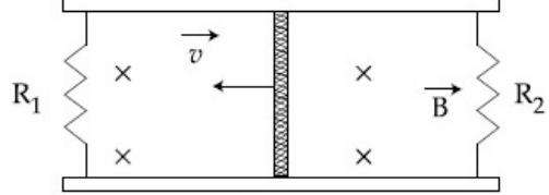
(A) The direction of induced current in the left part is anticlockwise and in the right part is clockwise.
