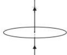
(A) the induced current in the ring is clockwise if the current through the wire is increasing.
