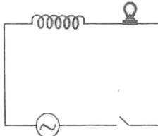
The switch is closed and after sometime, an iron rod is inserted into the interior of the inductor. As the iron rod is inserted, the glow of the light bulb:
