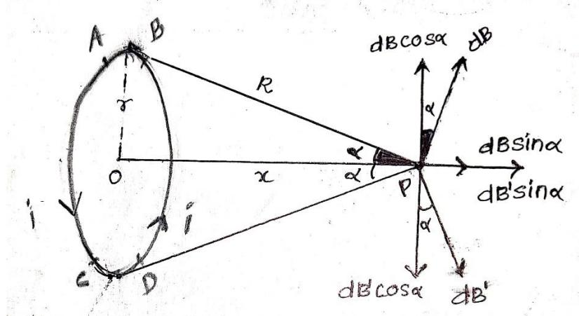
Consider a circular coil of 'n' turn and radius 'r' carrying a current I as shown in figure.
